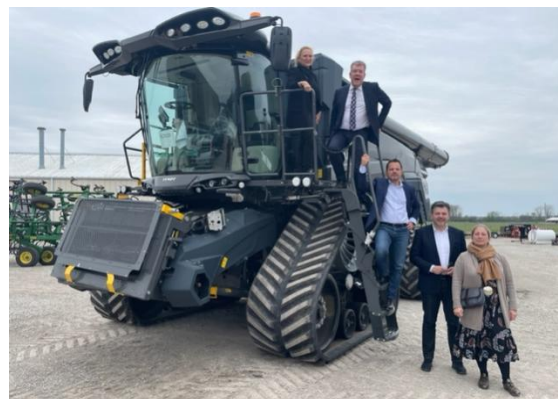
The delegation experiments with a geolocatable combine harvester, capable of producing precise maps of the field's yield, collecting and exchanging information on the harvest in order to optimally adapt the measures to be taken
